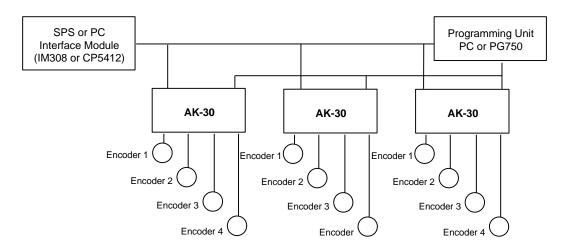
SSI Measuring System with Linear Absolute Path Sensors or Absolute Encoder
