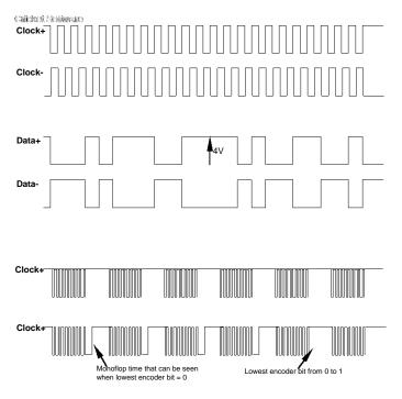
For safe data transfer, it is also possible to use encoders with a 28-bit checksum SSI. The checksum forms a BCH code, it is 15 bits long and has a Hamming distance of 6;: this means that it is always possible to detect up to five arbitrarily distributed errors or error bundles that can be up to 15 bits long. This allows very safe detection of faulty transfers, polarity-reversed clock or data lines or a missing encoder.
